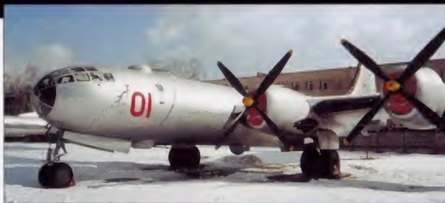
Above: Equipped with Kobalt blind bombing radar and powered gun turrets, the 'Bull' was the Soviets' first truly modern bomber aircraft.
